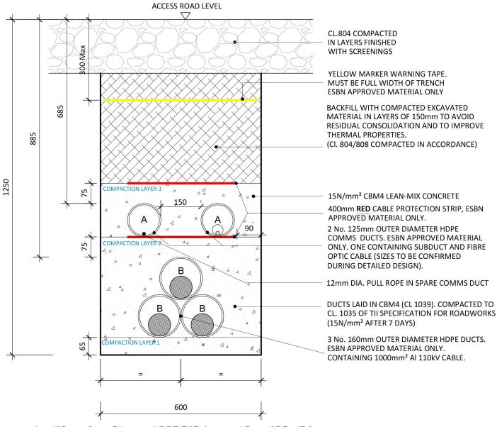
A = 125mm: Outer Diameter HDPE ESB Approved Duct, SDR=17.6 B= 160mm : Outer Diameter HDPE ESB Approved Duct, SDR=17.6
